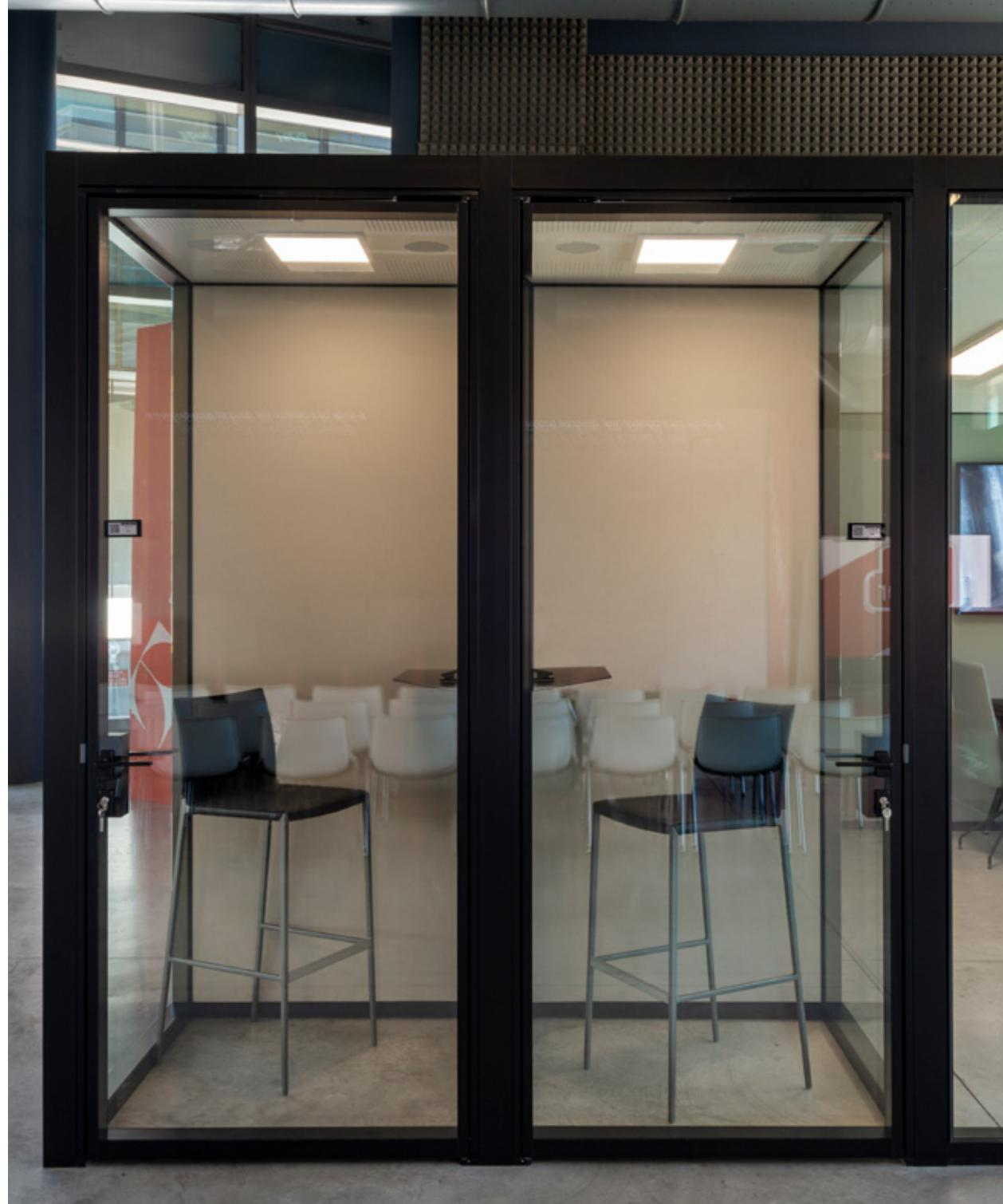
The LED lighting is dimmable while the silent and energy-efficient ventilation system ensures constant temperature, continuous air circulation and air purification. Blinds and LCD on/off area concealed within the glazed wall, while in the solid partitions runs cable routing and electrical controls for room reservation or video-conferencing monitors, switches or thermostats.
